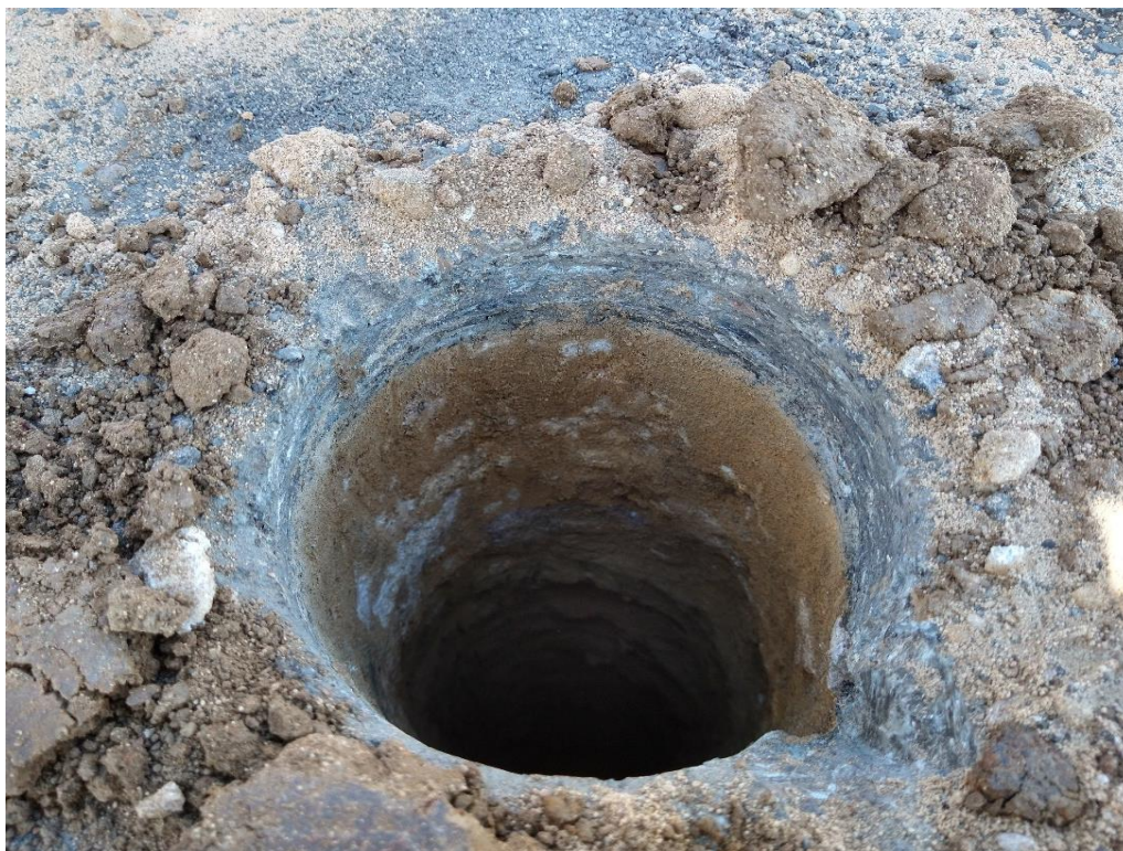
Photograph 3 - Visible layers of asphaltic concrete, sand (fill), and silty clay (natural) from borehole 110
