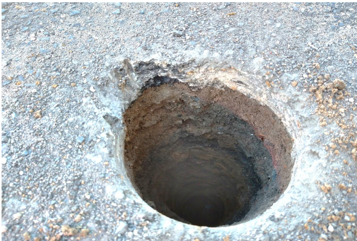
Photograph 8 - Visible layers of asphaltic concrete, roadbase, silty sandy clay (fill), and silty clay (natural) from borehole 121
