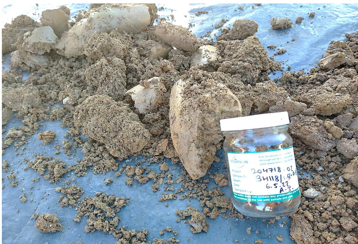
Photograph 6 - Natural clay material augered from borehole 118
